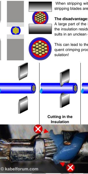
Error: Uncleanly cut, frayed insulation
