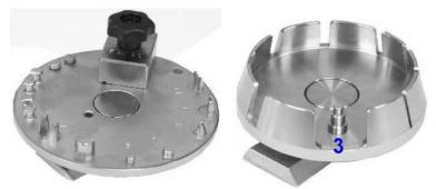
The picture on the right shows a special receptacle for wire-end ferrules: After insertion into the receptacle (1), a cover (2) is pushed over the wire-end ferrule. The ferrule cannot come out of the receptacle. The geometry of the receptacle prevents kinking. This means that it is not necessary to fix the ferrule by hand. An optimum measuring result is achieved.
