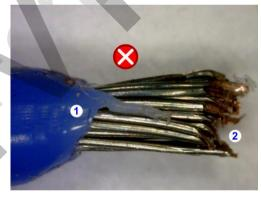
Error: (1) No clean cut due to straight and worn straight cutting blades in a wire stripper.
