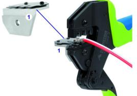
A correctly mounted positioning aid matched to the crimp contact is absolutely essential for creating a good crimp connection with hand crimping pliers.
