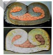
The crimp flanks are rolled in too far! Wrong assignment of crimp contact to conductor cross-section. The crimp contact is too large!
