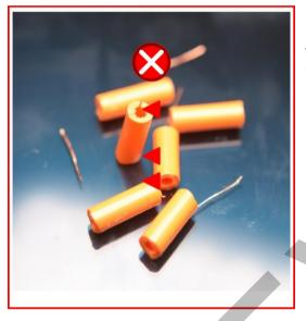
Effective control in manufacturing: When you find single, cut-off wire strands on the workstation or in the bin!
