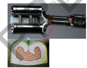
**open crimp barrel:** The crimp flanks support each other (A)
