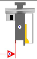
The surface (A) on the ram (1) is the reference surface for all assemblies in the crimping tool.
