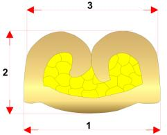
The crimp height (2) is an adjustable dimension in the processing tool. The crimp height is specified by the contact manufacturer depending on the conductor/cross section. As a non-destructive test, crimp height measurement offers reliable quality control during ongoing production.
