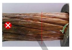
The color changes from a shiny orange-reddish shade to a matt dark brown surface, depending on the degree of oxidation (also called: passivating effect). This surface serves as a protective layer and prevents the penetration of oxygen or oxygen compounds such as water, thus stopping further corrosion and making copper very resistant to weathering.
