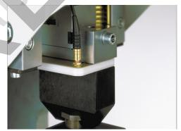
Top tool fixture of a RAM crimp force monitoring system (by Komax)
